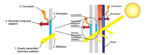
For well insulated buildings the main way that solar radiation enters a building is by passing through the glass in the windows. Glass is transparent to the shortwave visible light emitted by the Sun.
