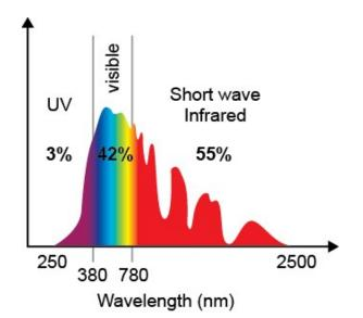
UV radiation = 320nm - 380nm Visible light = 380nm - 780nm Near Infrared (Shortwave IR) = 780nm - 2,500nm Thermal Infrared (Longwave IR) = 2,500nm - 25,000nm
